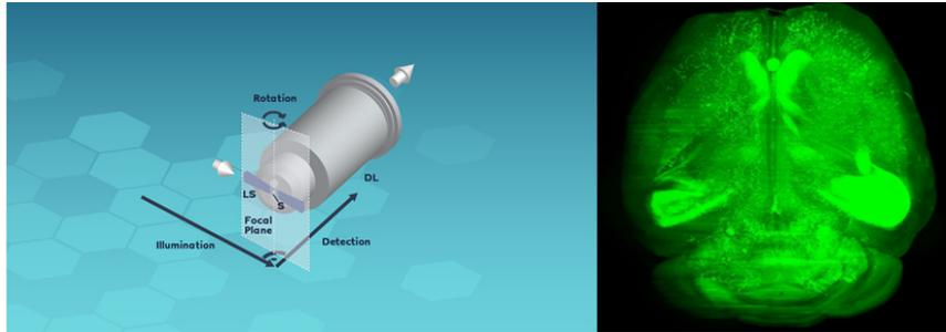
**Figure 14:** Light sheet microscopy. Left: Working principle. Right: Fluorescence image of a mouse brain taken with light sheet microscopy by fluorescence imaging. Credit: Fenerliabi11, Wikimedia Commons. Reproduced under the [Creative Commons Attribution-ShareAlike 4.0 International](https://creativecommons.org/licenses/by-sa/4.0/) license (CC BY-SA 4.0).
