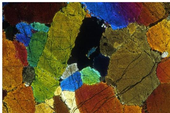
**Figure 9:** Polarization microscopy. Photomicrograph of olivine adcumulate, formed by the accumulation of crystals with different birefringence. Variations of thickness and refractive index across the sample result in different colors. *Credit: R. Hill, CSIRO.*
