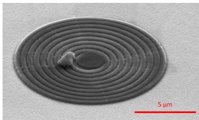
**Figure 18:** Scanning electron microscope image at 15,000 x magnification of a nanocrystal in a concentric polymer structure. Even fine details such as the pores
