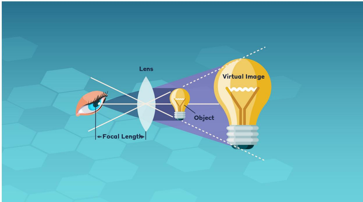
**Figure 2:** A single lens as a magnifying glass by creating a magnified, virtual image of an object placed close to it.
