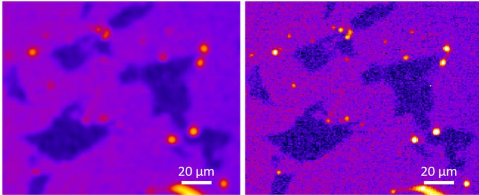
**Figure 17:** Image deconvolution. Left: Original fluorescence image. Right: Image after deconvolution, showing increased detail. *Credit: Author.*
