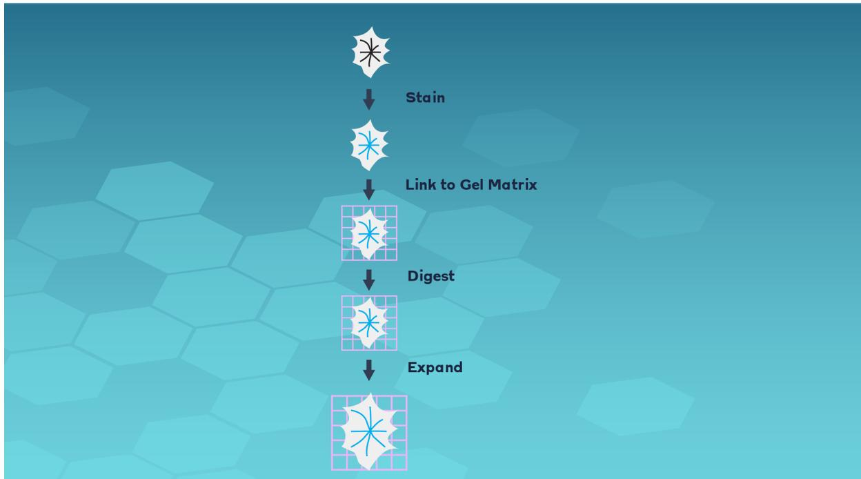
**Figure 16:** Sample preparation for expansion microscopy. A cell is first stained and then linked to a polymer gel matrix. The cell structure itself is then dissolved (digested), allowing the stained parts to expand isotropically with the gel, allowing the stained structure to be imaged with more detail.
