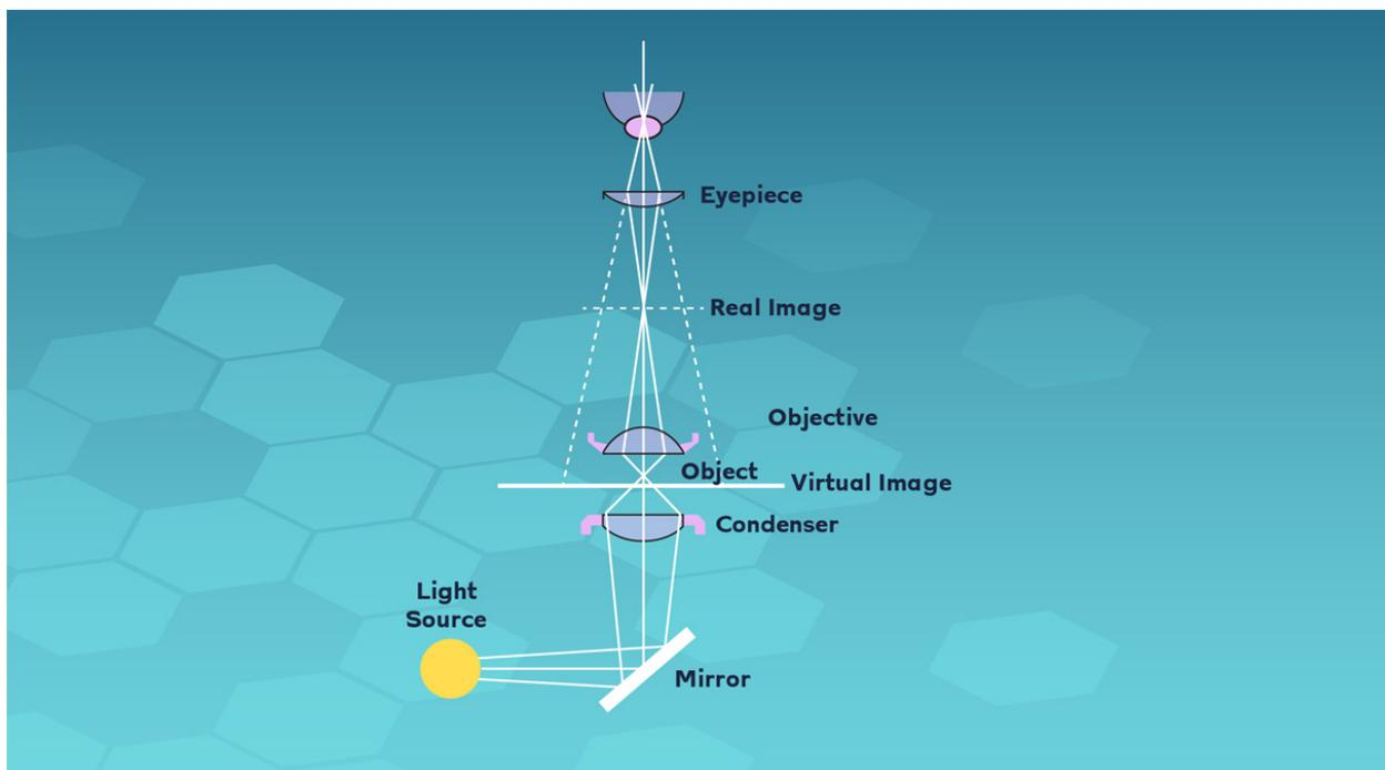
**Figure 1:** Basic compound microscope: Light from a source is focused onto the
