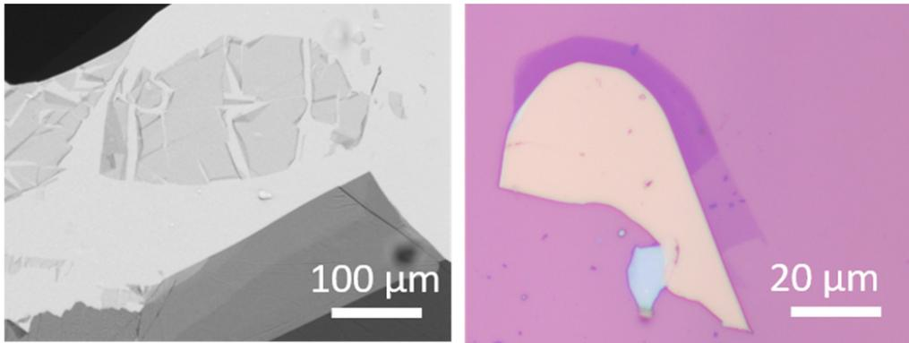
**Figure 5:** Bright field microscopy. Left: Transmission mode - flakes of graphite (dark grey) and graphene (lightest grey) as seen in a bright field microscope. Here, the difference in brightness seen on the image is proportional to the thickness of the graphite layer. Right: Reflection mode - flakes of graphene and graphite on a SiO<sub>2</sub> surface. Small surface contaminants are also visible. *Credit: Author.*
