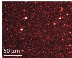
**Figure 12:** Confocal fluorescence image of single molecule fluorescence. Small spots correspond to fluorescence from individual molecules, while larger spots correspond to clusters of molecules. The fluorescence background here is much weaker than in a simple fluorescence microscope image, as seen by the dark areas between bright spots. *Credit: Author.*
