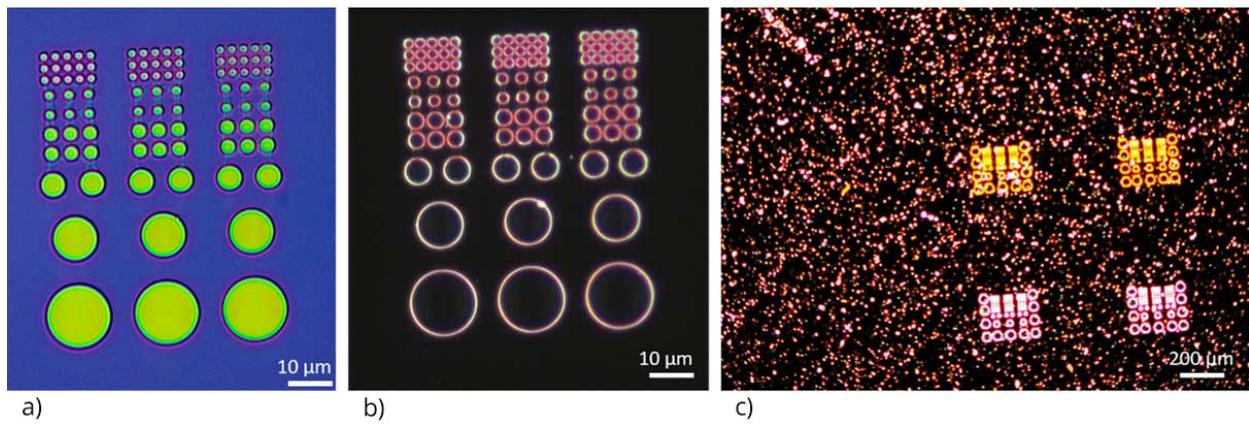
**Figure 6:** Bright field and dark field imaging. a) Polymer microstructure in bright field illumination. b) Dark field image of the same structure as in a), highlighting scattering from edges and surface contamination. c) Similar structures as in a) and b), covered by nanocrystals of 100-300 nm diameter. Only light scattered by the nanocrystals is observed, while the background light is strongly suppressed. *Credit: Author.*
